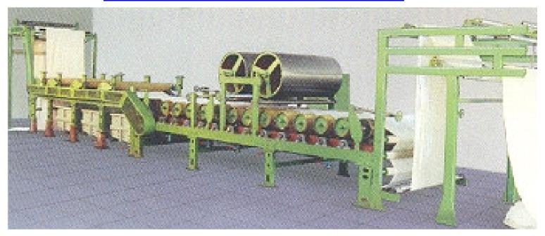
• Standard machine economically designed and equipped with two squeezers, one after impregnator, and the other after stabilizer
